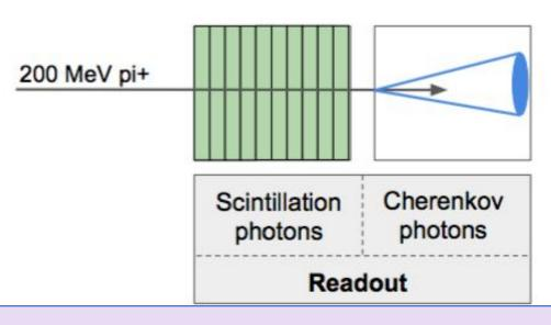
The HIBEAM/NNBAR Calorimeter prototype arxiv 2107.02147
