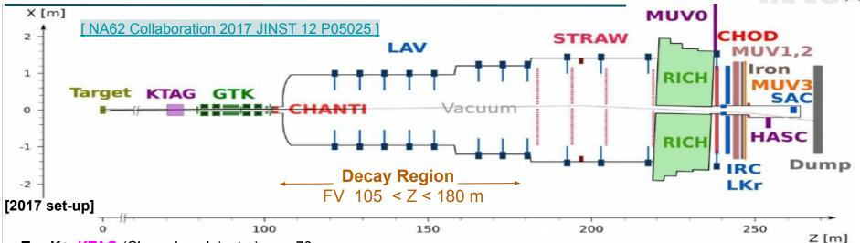
**Tag K+**: **KTAG** (Cherenkov detector),  $\sigma_t \sim 70 \text{ ps}$
