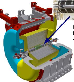
New calorimeters around the final focusing magnets
