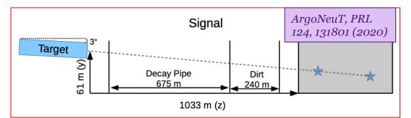
Searches for millicharged particles (blips along a straight line, pointing back to target)
