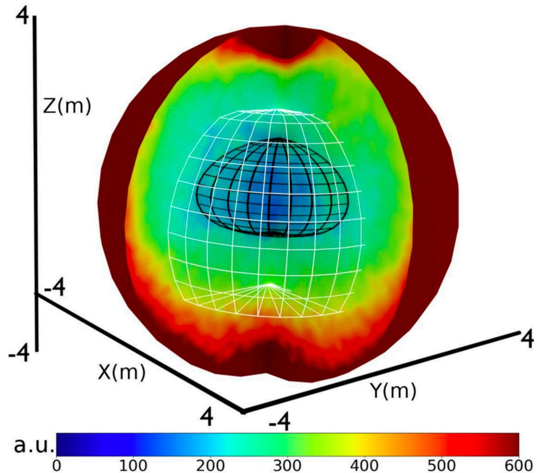
**Extended Data Fig. 5 | The low polonium field in the Borexino scintillator.** Three-dimensional view of the  $^{210}\text{Po}$  activity inside the entire nylon vessel (see colour code). The innermost blue region contains the LPOF (black grid). The white grid is the software-defined fiducial volume. a.u., arbitrary units.
