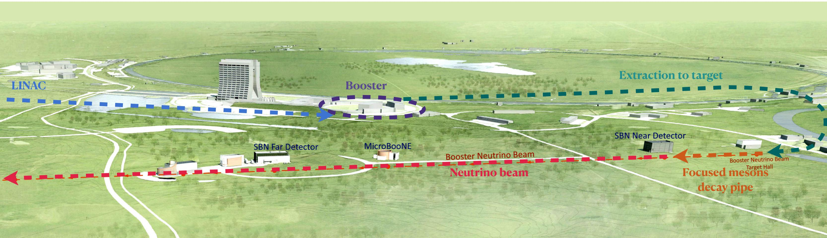
SBN **detectors** share the same nuclear target and similar technologies: liquid argon time projection chambers (TPCs). The detectors are strategically placed to look for neutrino oscillations at short baselines and low energy range along Fermilab's **Booster Neutrino Beam (BNB)**, which provides a highly pure source of either  $\nu_\mu$  or  $\bar{\nu}_\mu$ .
