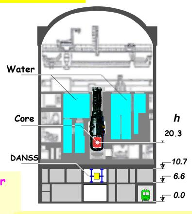
DANSS is installed on a movable platform under 3.1 GW WWER-1000 reactor (Core:h=3.7m, Ø=3.1m) at Kalinin NPP. ~50 mwe shielding => µ flux reduction ~6! No cosmic neutrons!
