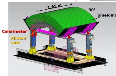
Pre demonstrator small prototype to be soon characterized at INFN-LNL
