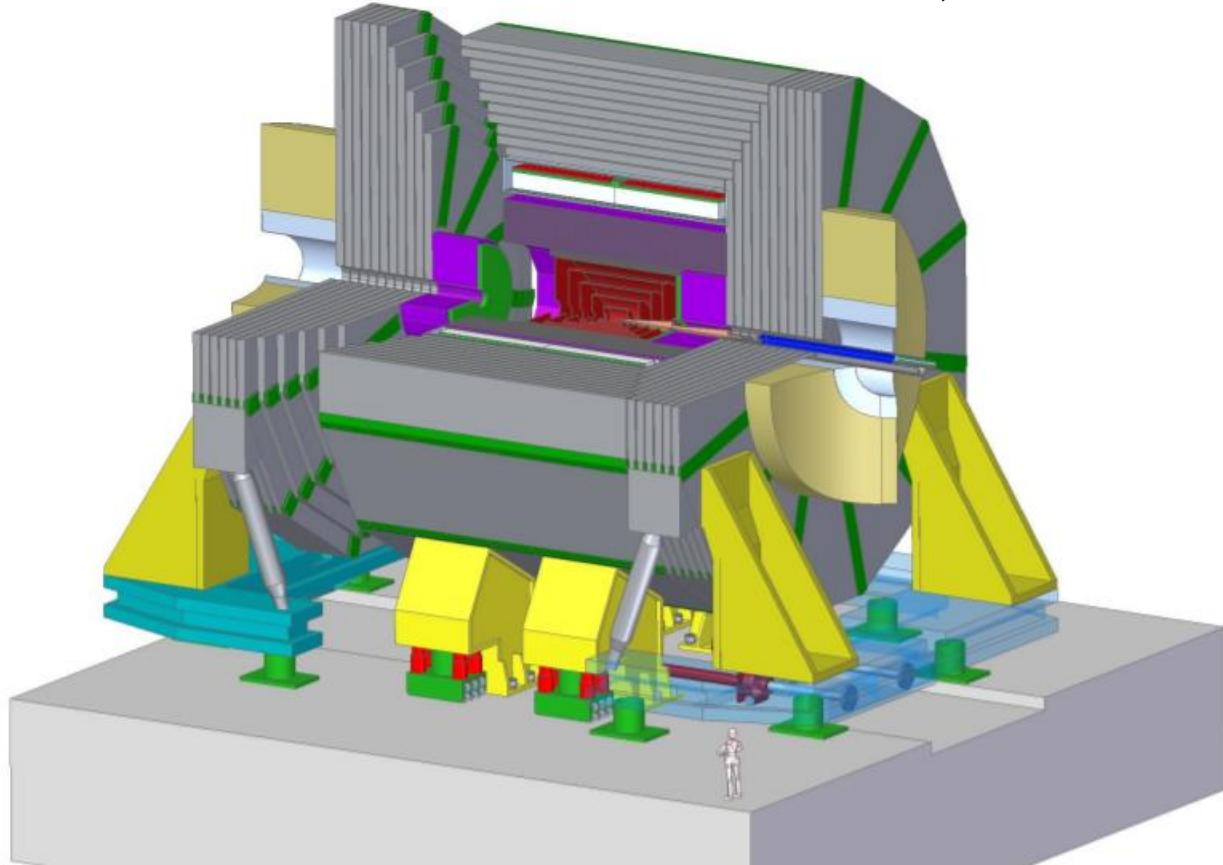
*A compact, cost-constrained detector designed to make precision measurements and be sensitive to a wide range of new phenomena*
