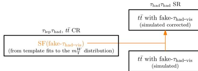
Figure 6: Schematic depiction of the fake- $\tau_{\text{had-vis}}$  scale-factor method to estimate  $t\bar{t}$  background with fake- $\tau_{\text{had-vis}}$  in the  $\tau_{had}\tau_{had}$  channel.
