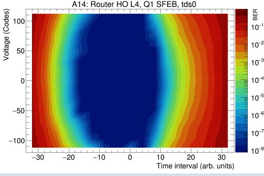
Classic eye: overlapping of many signal waveforms Statistic eye: BER as a function of sampling time and voltage
