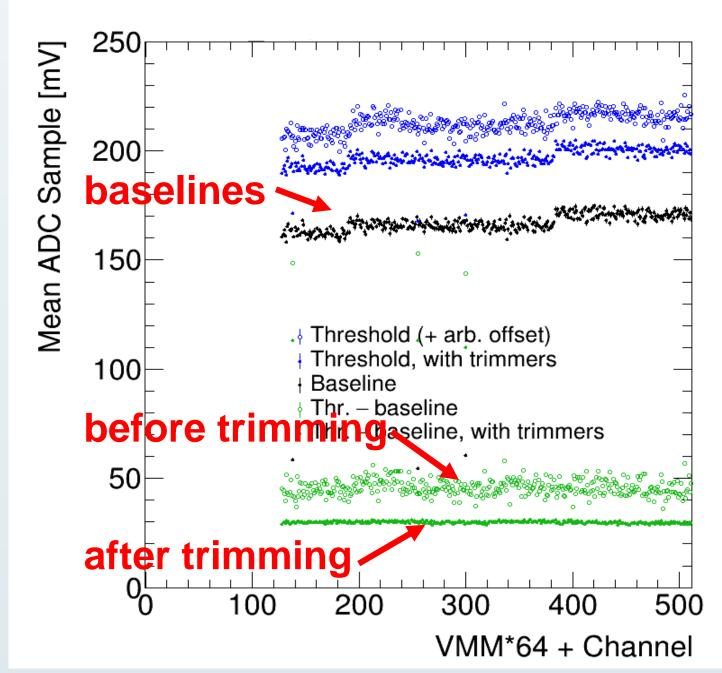
Set global threshold to entire VMM and add trimmers to equalize threshold baseline value for above each individual channels.
