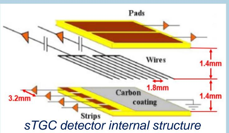
The sTGC and the MM can both provide complementary trigger and tracking information. Given its single bunch crossing identification ability, the sTGC will be used as the primary trigger detector. It has 3 types of readout channels, among which only pads and strips are used for Level-1 triggering.
