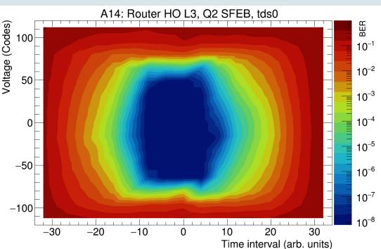
Statistic eyes with BER cutoff at 10<sup>-8</sup>. Eye on the right indicates larger signal attenuation and more time jitter than the eye on the left since the height and width of the eye are smaller.
