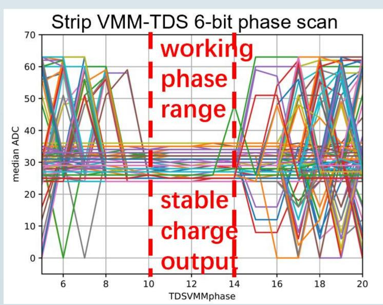
Strip-TDS uses a common clock to read VMM 6b ADC from all channels. A clock phase scan is performed to determine the range that has stable output for all channels.
