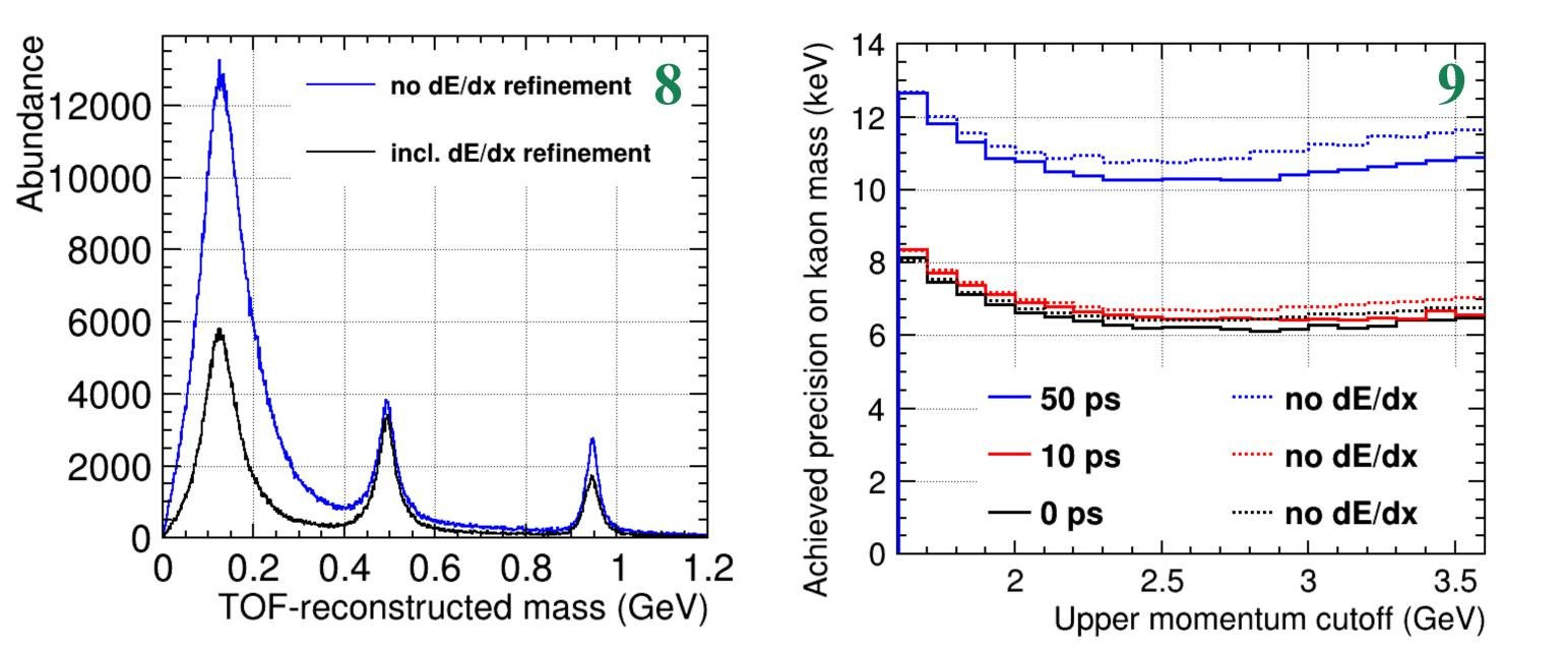
Translate  $\beta$  into mass, use dE/dx to reduce background, fit mass. ILC 2 ab<sup>-1</sup> @500 GeV gives stat. precision of 10 keV, better than current PDG uncert. of 13 keV.
