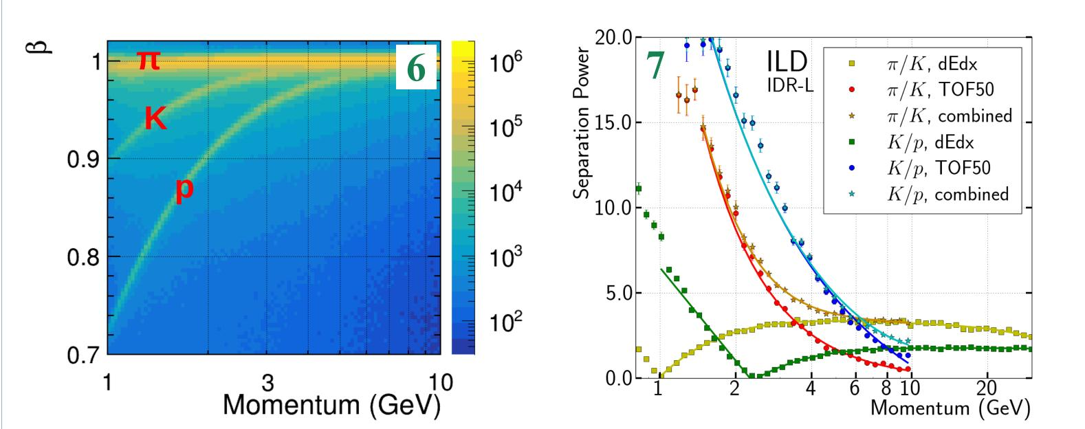
Measure timing from IP to ECal entry point  $\rightarrow$  velocity  $\beta$ . ECal time: average of 10 hits closest to track. Get separation power, covers dE/dx blind spots.
