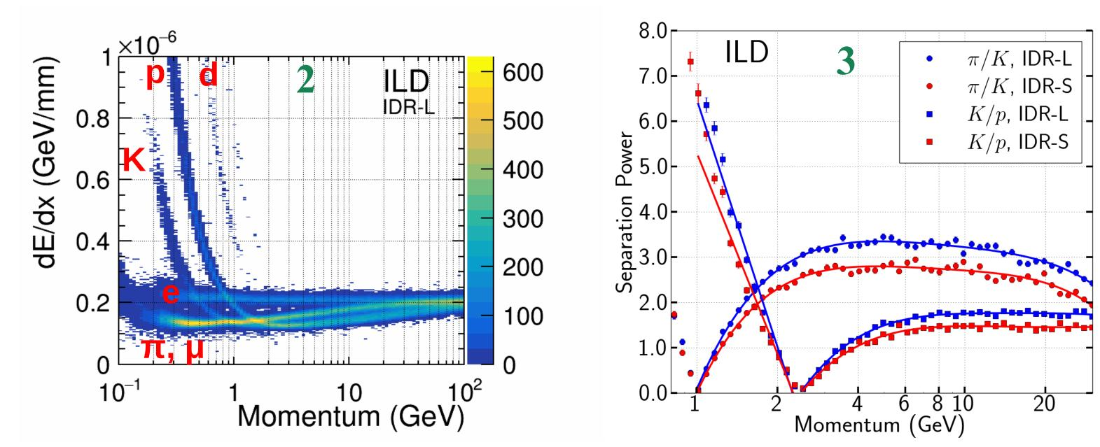
Tracks in the TPC have up to 220 hits, measure energy loss/flight distance (70% trunc. mean). Calculate distance between Bethe-Bloch bands: separation power.
