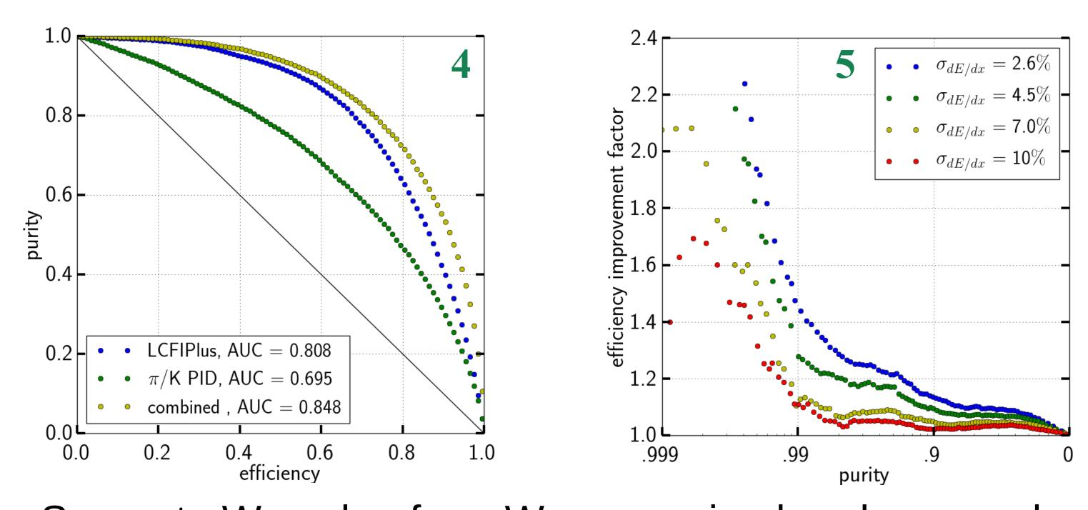
Separate W  $\rightarrow$  d+u from W  $\rightarrow$  s+c via abundance and momentum of kaons vs. pions, compare to default flavour tag. Helps determination of CKM matrix, in particular  $V_{cs}$ .
