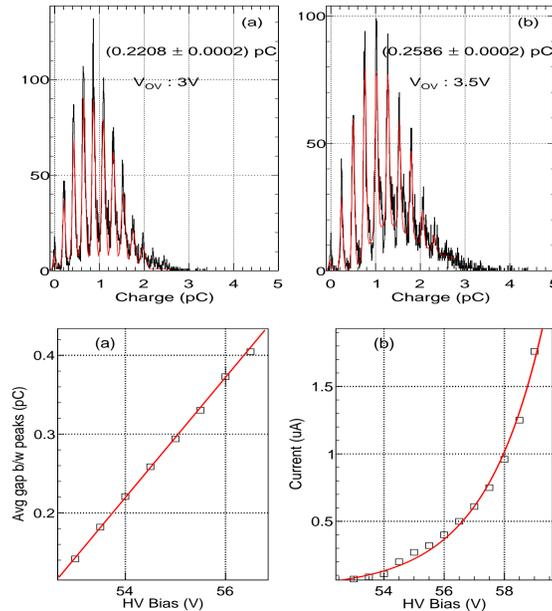
Good linearity of gain with  $V_{ov}$ . Dark current increases exponentially with  $V_{ov}$ , where  $V_{br} = 51.0$  V.
