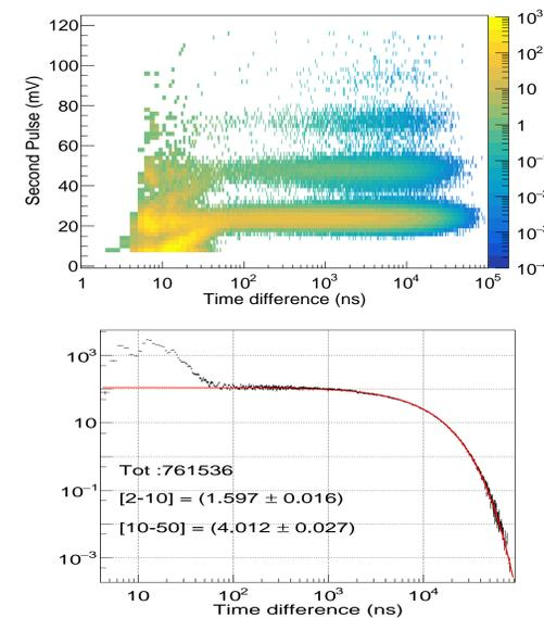
Events due to afterpulse and crosstalk can be seen clearly. Rates have been calculated by taking the difference between the actual values and the fit values by extrapolation.
