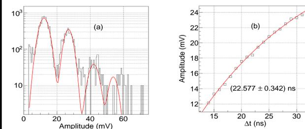
The distribution (a) is fitted with individual four Gaussian functions, 2nd and fourth are for the peak of after pulse and the distribution (b) is fitted with :
