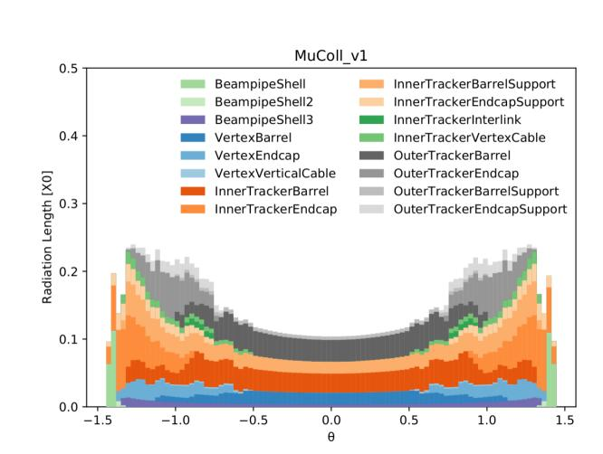
ACTS simplifies the track propagation through the detector by using a binned material map based on a GEANT simulation.
