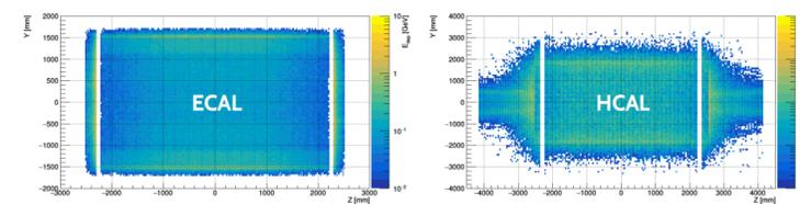
**Electromagnetic Calorimeter (ECAL):** 40 layers W absorber and silicon pad sensors, 5x5 mm<sup>2</sup>
