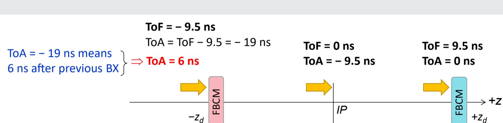
BIB simulations using CMS reconstruction SW framework with input from FLUKA were carried out. Using time binning of 0.78 ns at 40 MHz rate will allow to identify incoming BIB @ ToA = 6 ns with a clear signature.
