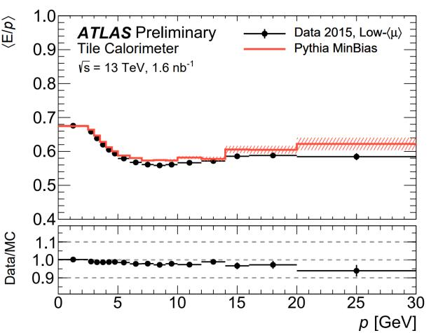
linearity. Expected to be < 1 due to noncompensating nature of the calorimeter. Data and Monte Carlo simulations agree within 5%.
