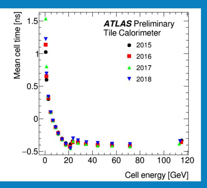
The Tile Calorimeter plays an important role in the ATLAS detector. Several calibration systems guarantee the stability of the cells response. They allow to control several parts of the readout chain and provide calibrating
