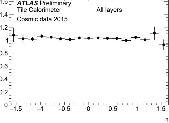
The ratio of energy measured by TileCal to the track **momentum** (E/p) is used to evaluate **uniformity** and
