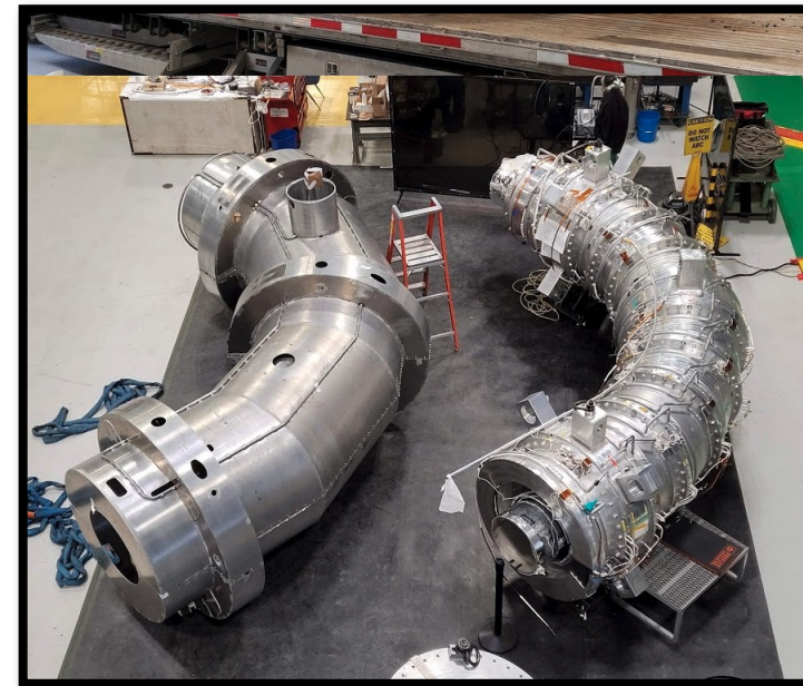
Tsu cold mass and thermal shield
