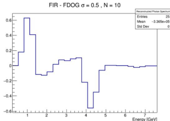
**Figure:** Response of the deconvolved spectrum to the FDOG filter with  $N = 10$  windows and  $\sigma = 0.5$ . The minimum value of this function locates the first order Compton edge.
