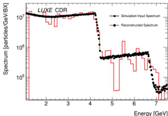
**Figure:** Comparison of the deconvolved spectrum (red) with the original input photon spectrum (black). First order Compton edge clearly visible at 4.2 GeV.
