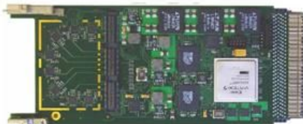
AMC 105 MS/s 8 Ch 14 bit ADC
