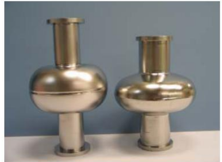
Figure 1: Left: 60 mm aperture re-entrant cavity; Right: 70 mm aperture TESLA cavity.
