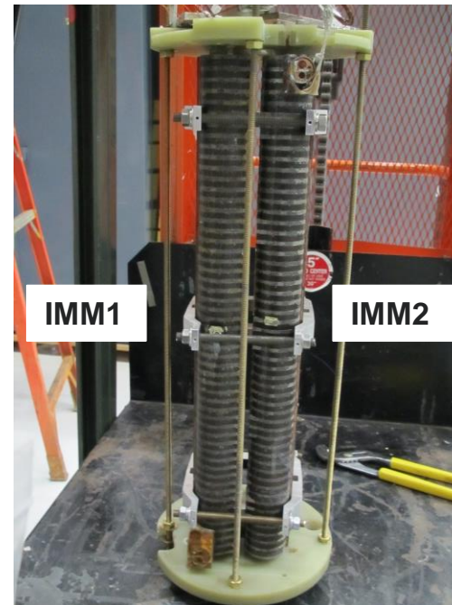
IMM1 and IMM2 undulator test
