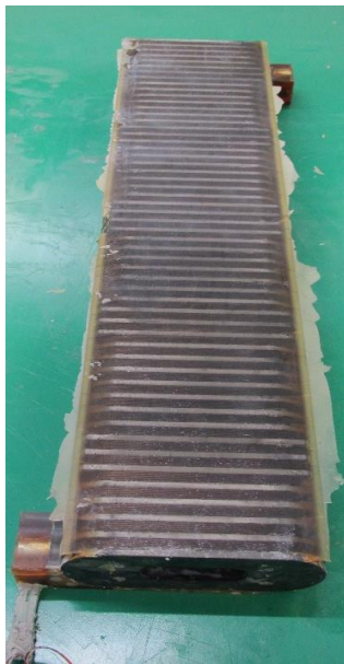
0.5 m long magnets after epoxy impregnation
