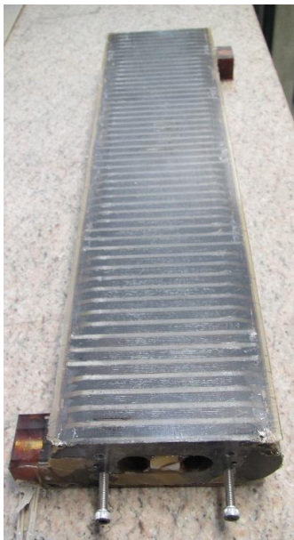
0.5 m long magnets after epoxy impregnation
