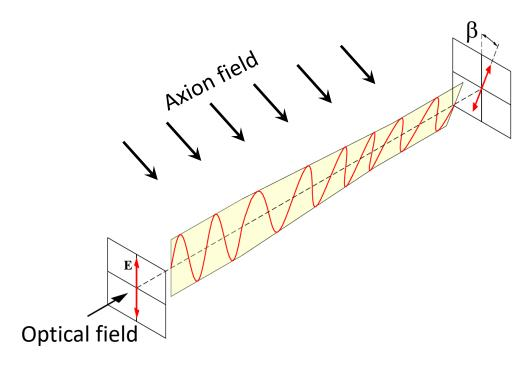
A rotation of the polarization state (converting a fraction of  $\updownarrow$  to  $\longleftrightarrow$ )
