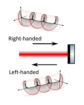
Or horizontal and vertical polarization have 180 degree phase difference after reflection
