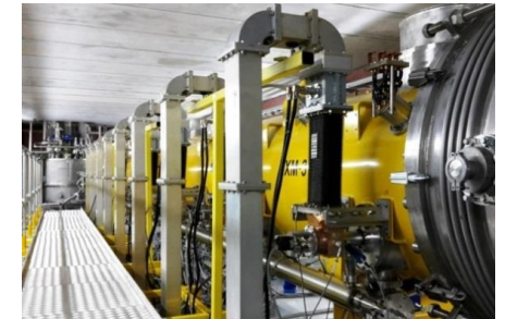
long pulse / CW operation of slightly modified XFEL type accelerator modules
