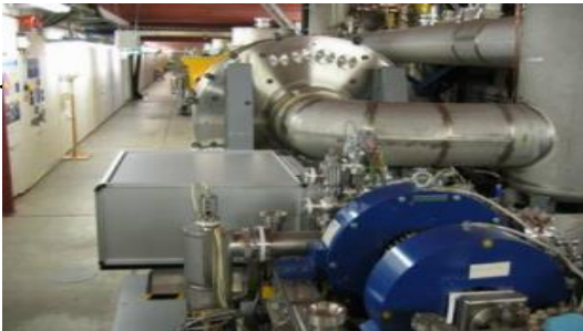
Normal conducting 1.3 GHz RF gun Ce 2 Te cathode / 3 injector lasers
