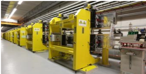
FLASH2 variable gap undulators
