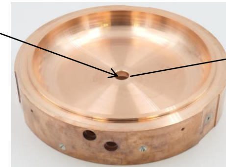
Final machined cathode body of Gun5
