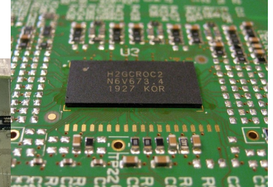
HGCROC(V2) on the back side of the tileboard
