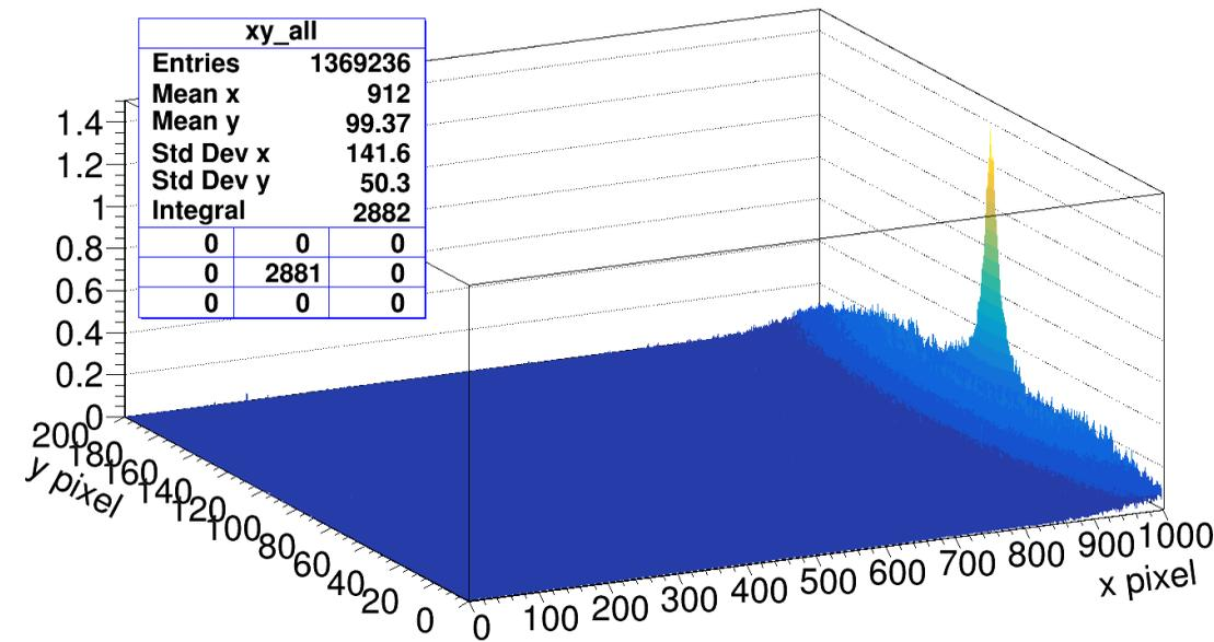
Back to QGSP\_BERT. Deposition in energy of IP Scintillation Screen [Z dimension in GeV]. Including these particles means a modest shift in the integral of energy deposited in the entire screen [GeV] from 2667  $\rightarrow$  2882.
