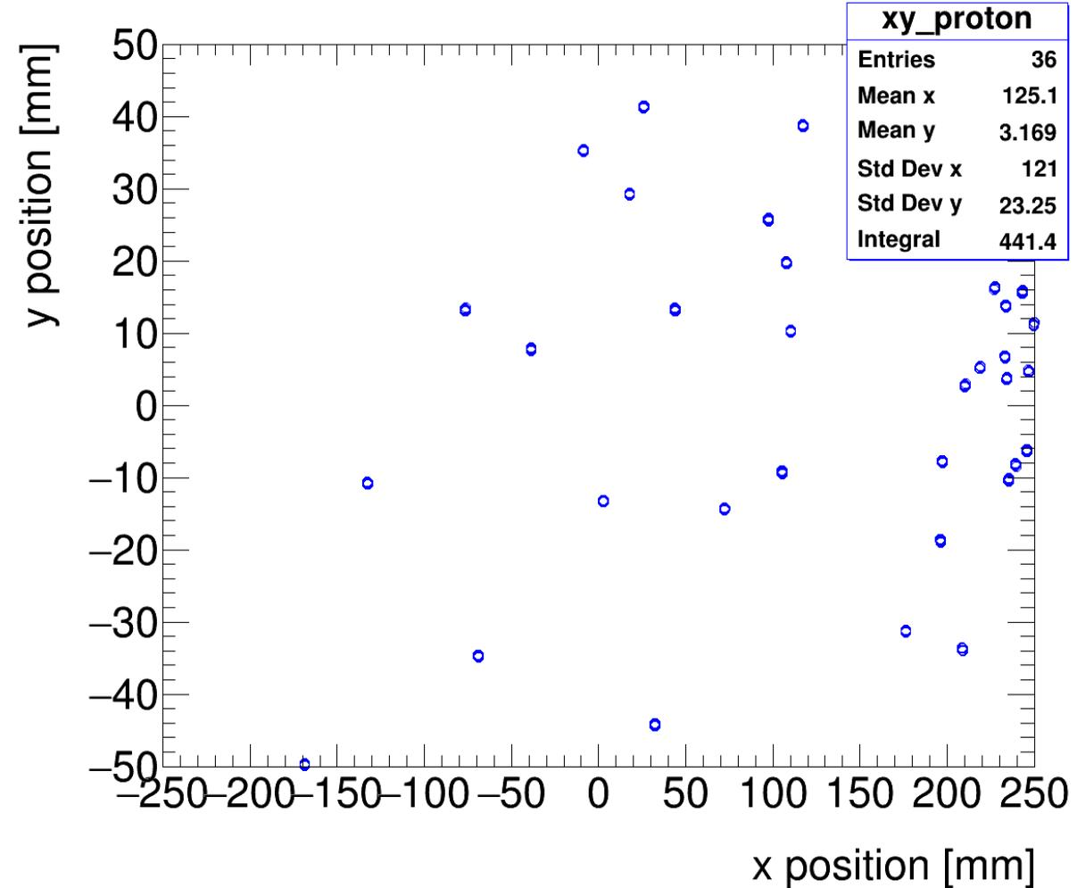
A beam-line-centred distribution (mean x close to far right). XY position is again relative to centre of screen.
