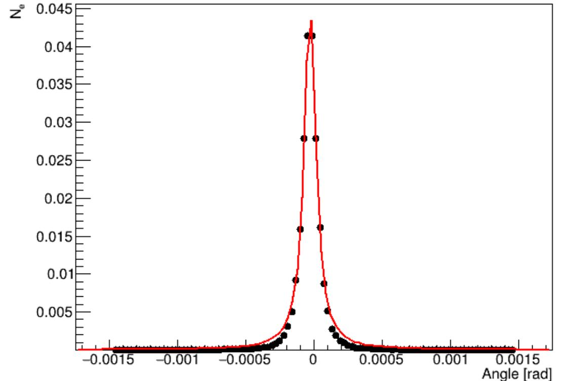
$$f(x; x_0, \gamma) = \frac{A}{\pi\gamma} \left[ \frac{\gamma^2}{\gamma^2 + (x - x_0)^2} \right]$$
