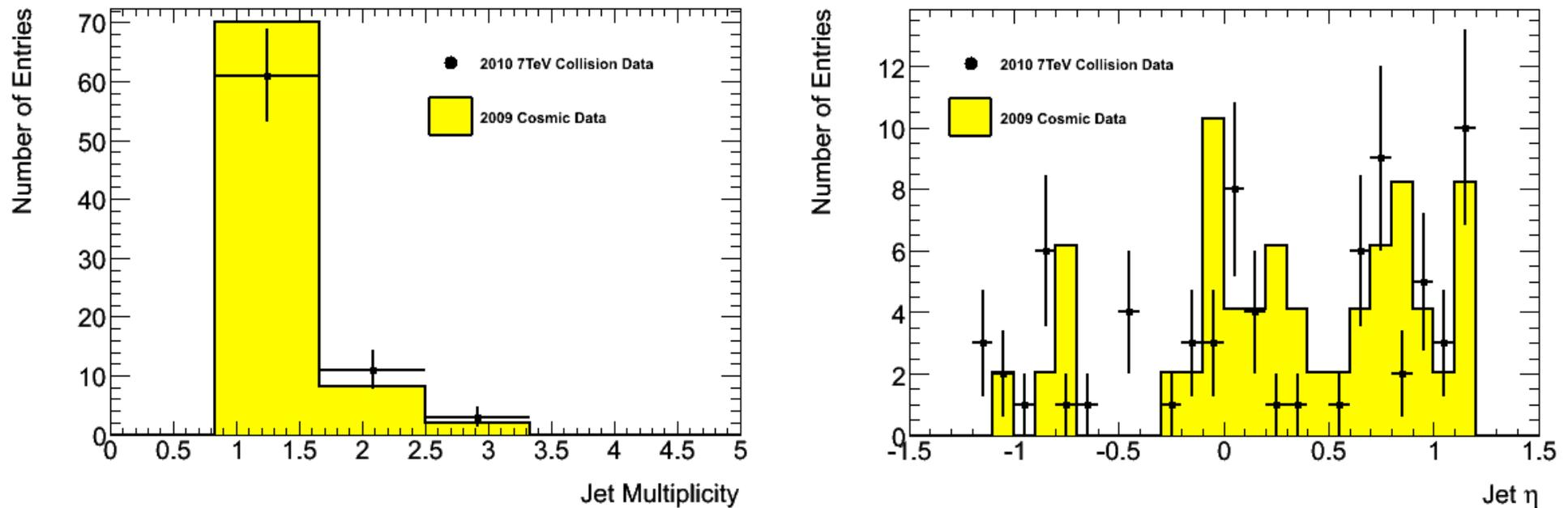
Figure 1: Jet variables plotted for the empty bunch triggers in 7 TeV collision data (black points) compared with 2009 cosmic data (filled histogram). We demand that all cleaning cuts are applied and that  $n_{90} > 3$ . We further require that there are zero reconstructed muon segments, that there be a leading jet with energy greater than 50 GeV and situated within  $|\eta| < 1.2$ . The jet multiplicity (left) and leading jet  $\eta$  (right) are plotted.
