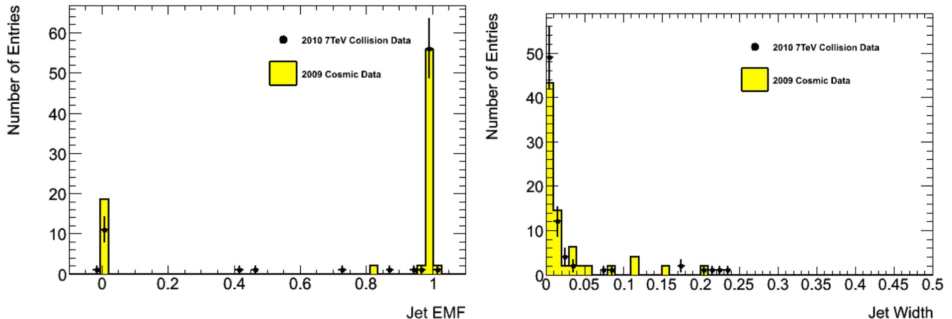
Figure 2: Jet variables plotted for the empty bunch triggers in 7 TeV collision data (black points) compared with 2009 cosmic data (filled histogram). We demand that all cleaning cuts are applied and that  $n_{90} > 3$ . We further require that there are zero reconstructed muon segments, that there be a leading jet with energy greater than 50 GeV and situated within  $|\eta| < 1.2$ . The leading jet electromagnetic fraction (left) and leading jet width (right) are plotted.
