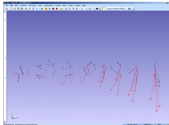
Figure 3: difference between adjusted and coarse coordinates for network 2 using 7 instruments, black=PANDA, red=SA
