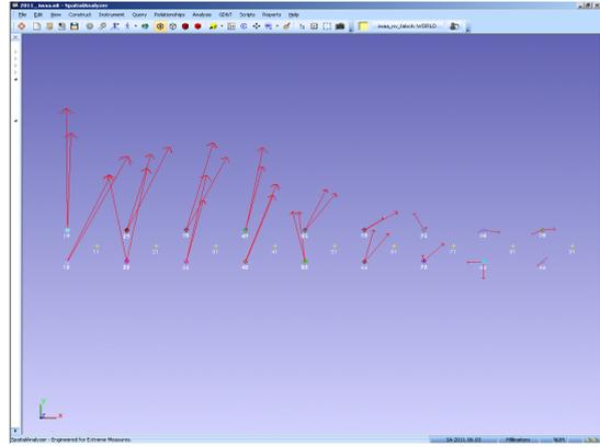
Figure 5: difference between adjusted and coarse coordinates for network 2 using 9 instruments (SA only), instruments imported in reverse order
