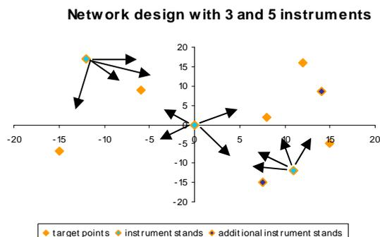
The ‘true’ observations  $\tilde{L}$  for the instruments were calculated and distorted by the described method. The distorted observations  $L$  are imported into PANDA and Spatial Analyzer. The error-free coordinates of network points were also imported and used as coarse coordinates to locate the instruments in SA and as initial values for the vector of unknowns  $X_0$  in PANDA.
