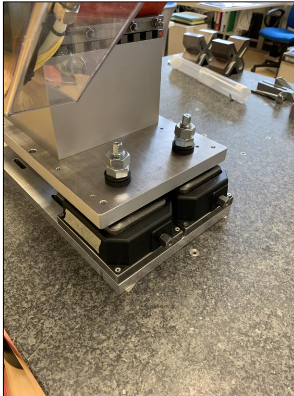
Levelling wedges installation
