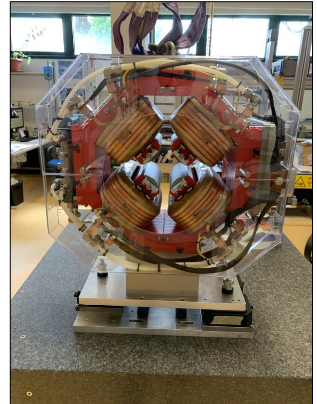
Mock up of the magnet support system
