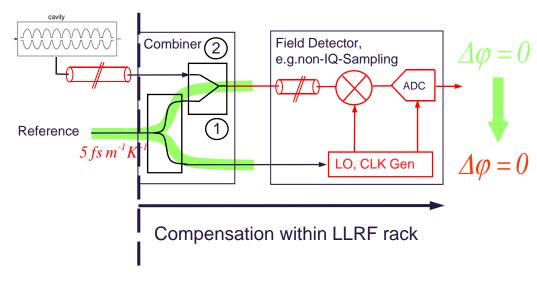
Injected reference Cavity signal and calibration Measurement
