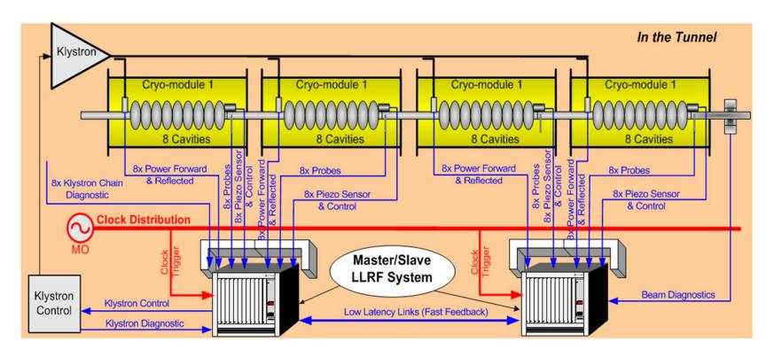
Driving Argument — Short pickup cables for low drifts (10fs/m/K) and prevent crosstalk from high power cables
