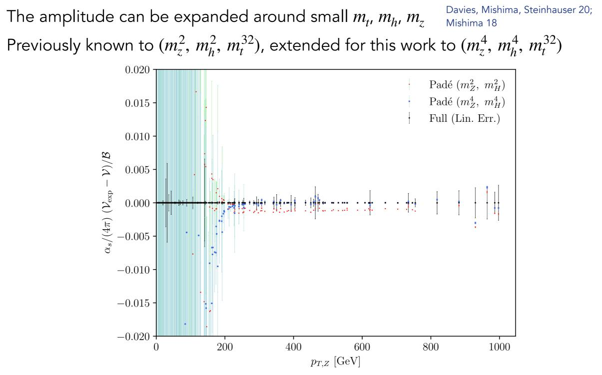
Find **acceptable** agreement for  $p_{T,Z} \ge 150$  GeV (<2.8% difference) Switch from the full numerical result to Padé result at this point
