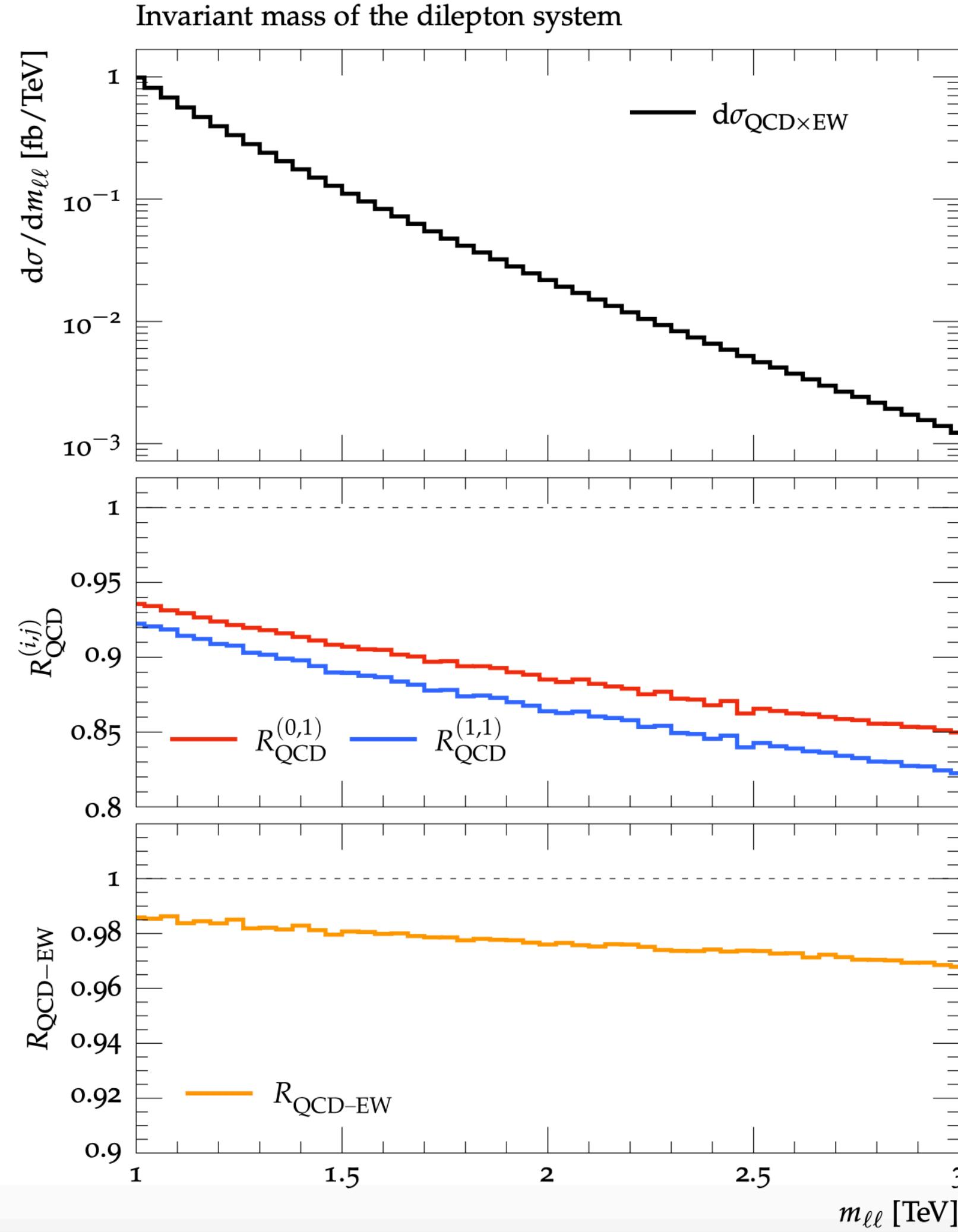
$$R_{\text{QCD}}^{(0,1)} = \frac{d\sigma^{(0,0)} + d\sigma^{(1,0)} + d\sigma^{(0,1)}}{d\sigma^{(0,0)} + d\sigma^{(1,0)}}$$
