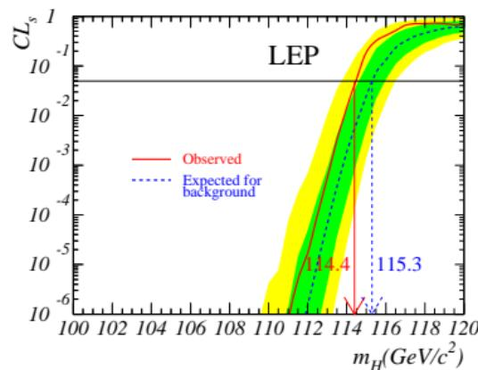
Confidence level  $CL_s$  for the signal+background hypothesis. The intersection of the observed limit with the horizontal  $CL_s = 0.05$  line determines the 95% CL lower mass limit.
