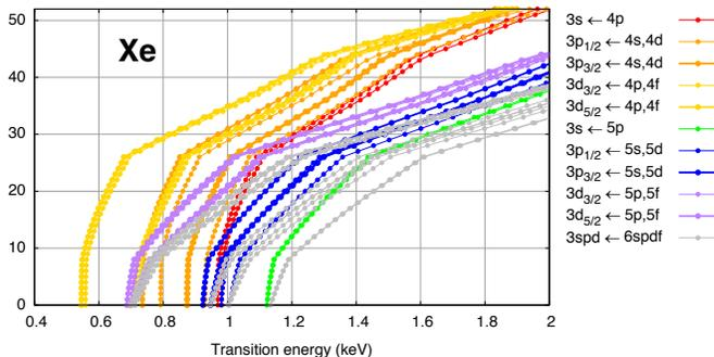
Fig. 1. A prediction of emission energies for radiative transitions to the M shell in Xe.
