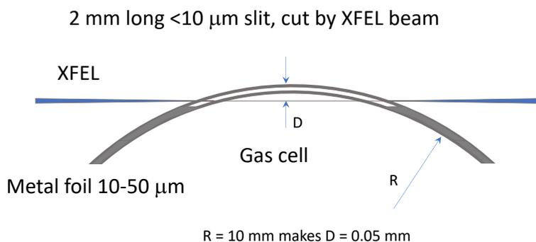
Fig. 2. Schematics of the new gas-cell concept.
