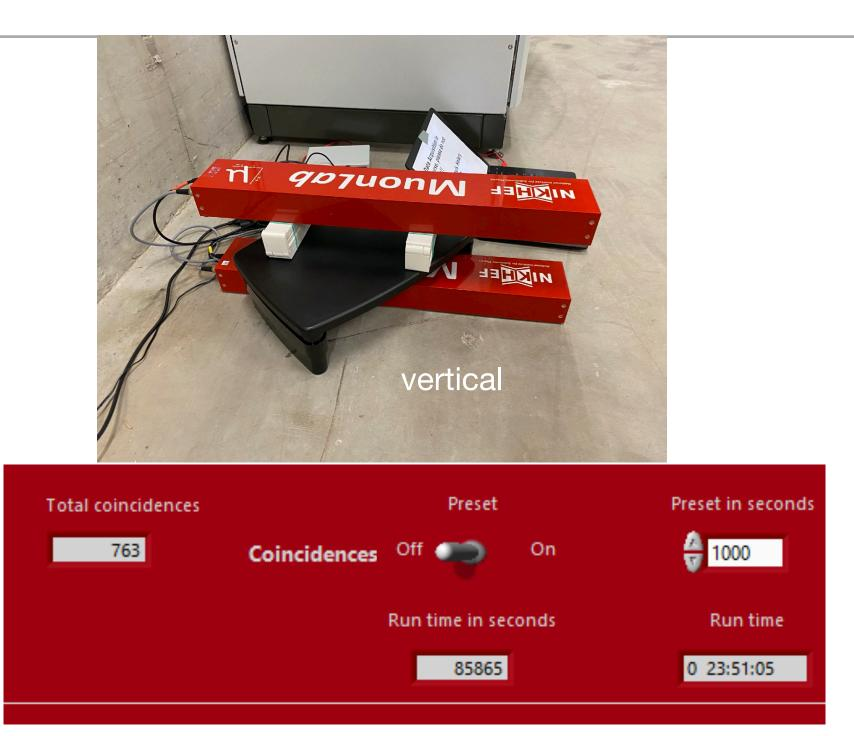
corrected time: total vertical run: 37min 4s. (763 coincidence in 2224s -> 0.343+-0.013 cosmics/sec).
