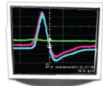
Bunch structure measured using beam pickups
