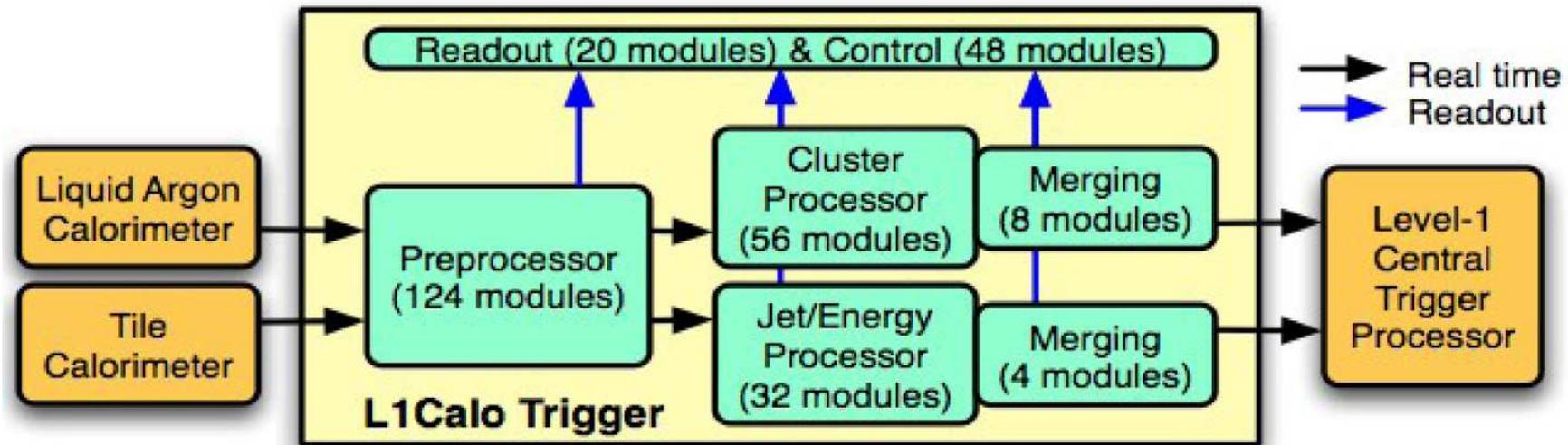
Fixed latency, pipe-lined, hardware based system using custom electronics
