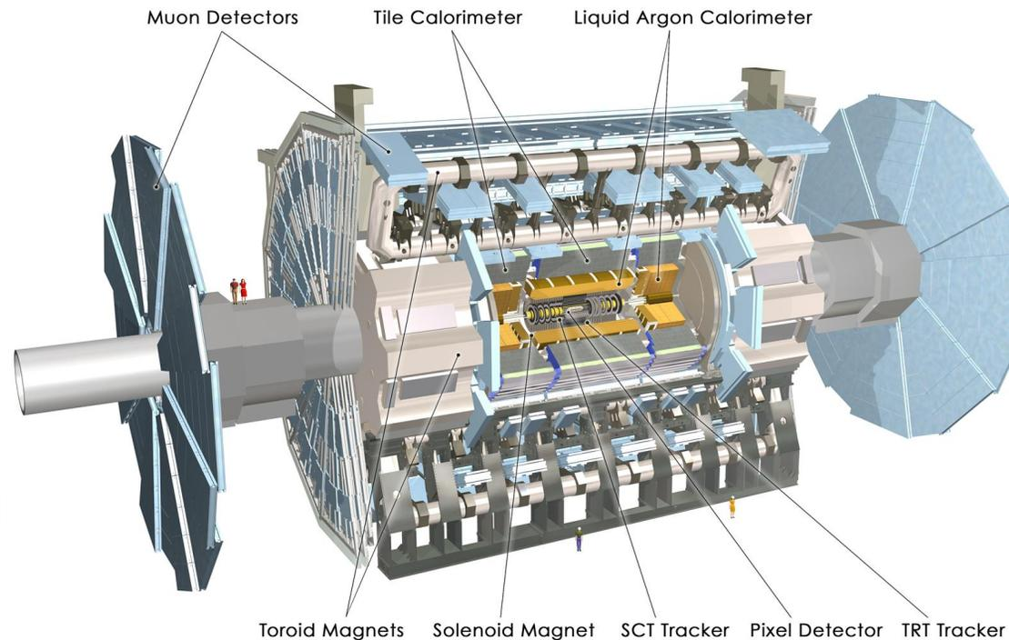
The ATLAS calorimetry consists of
