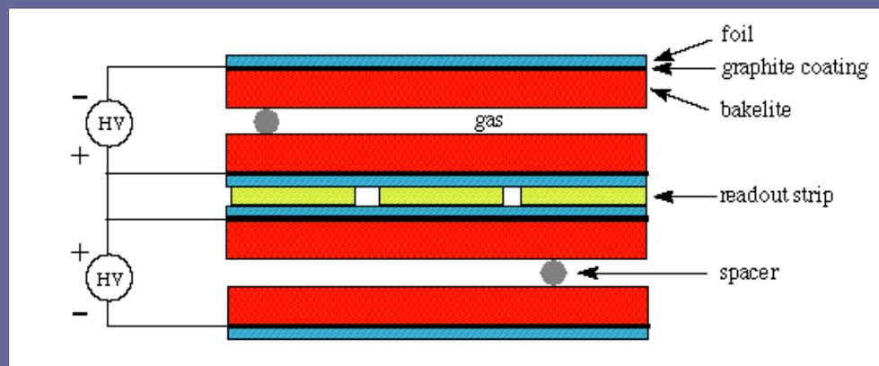
Gas gap needs constant width. Signal in pick up electrodes
