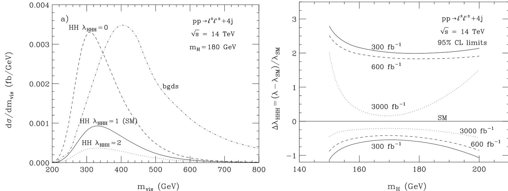
(a) The  $m_{vis}$  distribution of the signal for  $pp \rightarrow HH \rightarrow W^+W^-W^+W^- \rightarrow \ell^\pm \ell'^\pm + 4j + E_T^{\text{miss}}$  and  $m_H = 180$  GeV at the LHC the SM, for  $\lambda_{HHH}/\lambda_{SM} = 0$  (dashed); 1 (solid) and 2 (dotted), as compared to backgrounds (dotted).
