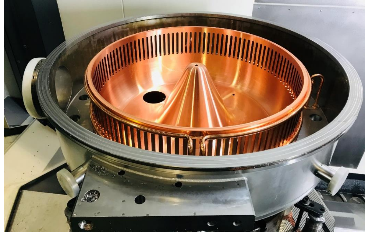
Cathode assembly after final machining
