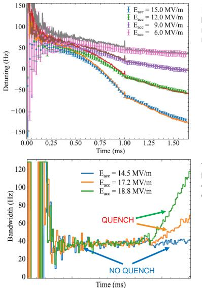
Detuning validation between reference measurement and model-based estimation
