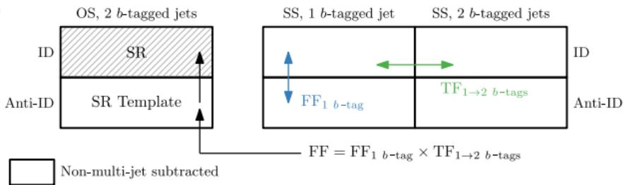
Figure 5: Schematic depiction of the combined fake-factor method to estimate the multi-jet background with fake- $\tau_{\text{had-vis}}$  in the  $\tau_{\text{had}} \tau_{\text{had}}$  channel. Backgrounds with true- $\tau_{\text{had-vis}}$  that are not from multi-jet events are simulated and subtracted from data in all the control regions. This is indicated by "Non-multi-jet subtracted" in the legend.
