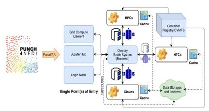
providing unified access and ensuring an efficient utilisation. These opportunistic compute resources can e.g. access huge storage resources through dynamic XRootD-based data caches. These have been developed and tested in an ErUM-Data pilot project and will provide access to a planned virtual data centre concentrating data storage inside a few large data centres interconnected by high-speed network links.
