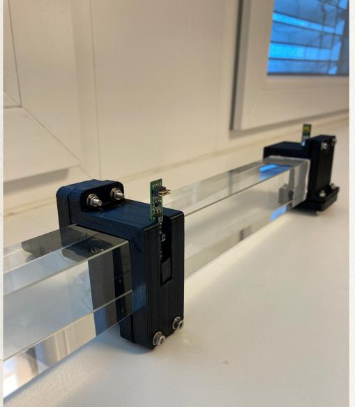
In previous measurements with and w/o wrapping we didn't see the difference when shining LED through the crystal's end which is explained by the total internal reflection (LG refraction index is 1.65, angle 37 grad or 53 grad with respect to surface.) 5 locations: close to PMT, 10 cm, 20, 30 cm and 38cm LED voltages in the range 7.0-9.0 V
