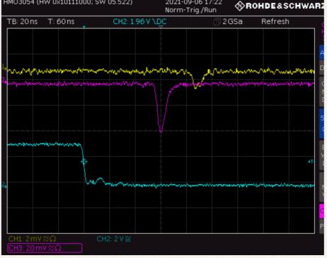
Both crystals see signal from LED when we read out 2 crystals laying in light tight box;
