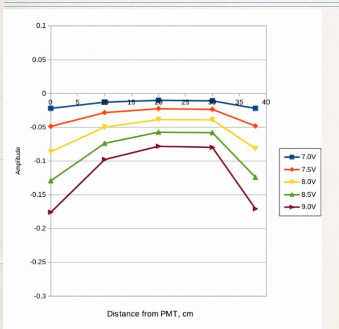
Signal is the lowest in the middle of the crystal, while the highest when the LED is located either close to PMT / or at the end of the block. This is due to the fact that light is leaking from the sides.
