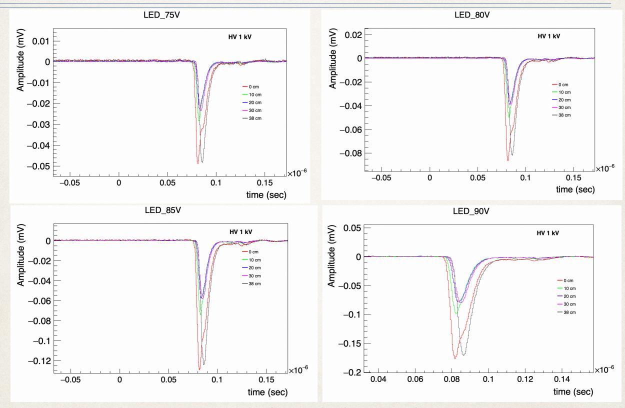
The displayed pulse shapes are obtained from averaging 50 recorded waveforms per LED voltage.
