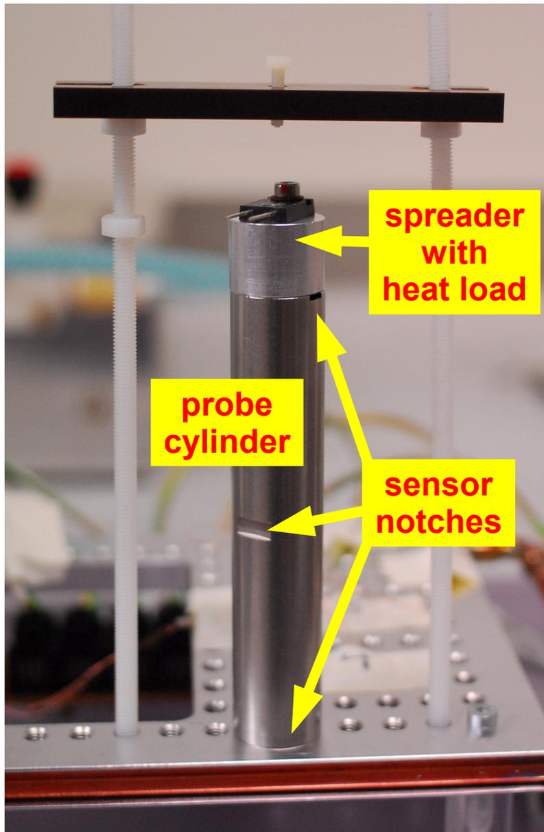
Measuring thermal conductivity of various material probes -
