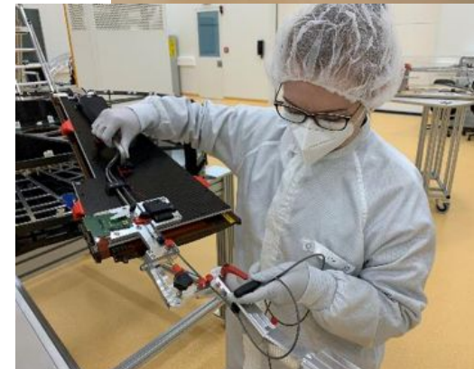
Petal insertion at DESY using insertion tool and super-frame
