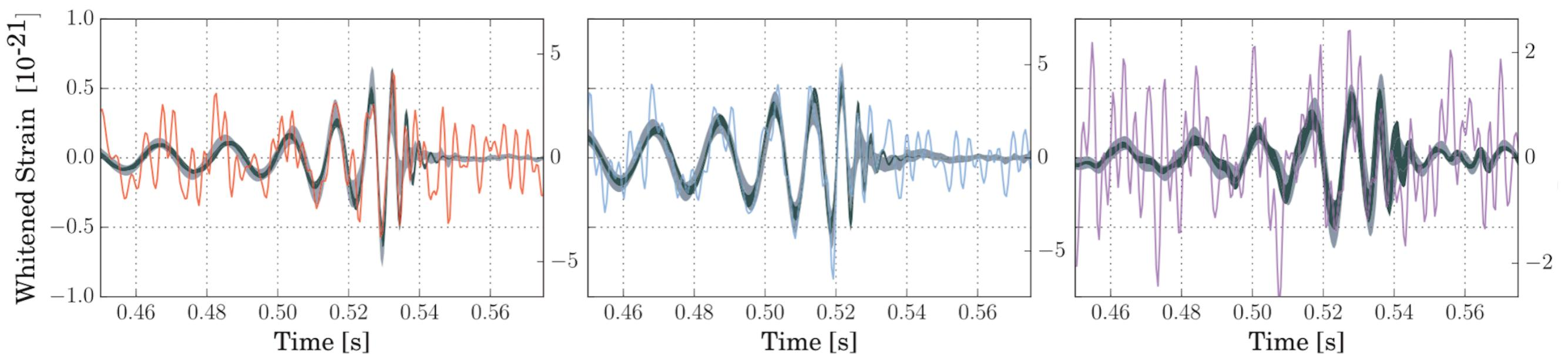
Exponentially damped sinusoidal waves: Quasi Normal Modes (QNM)
